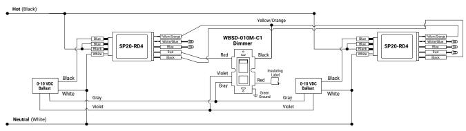
Note: DLC-PD-DIM can be added to this configuration to provide continuous daylighting of the 0-10V loads. The device with the lowest 0-10V value will hold the lighting at that level.
